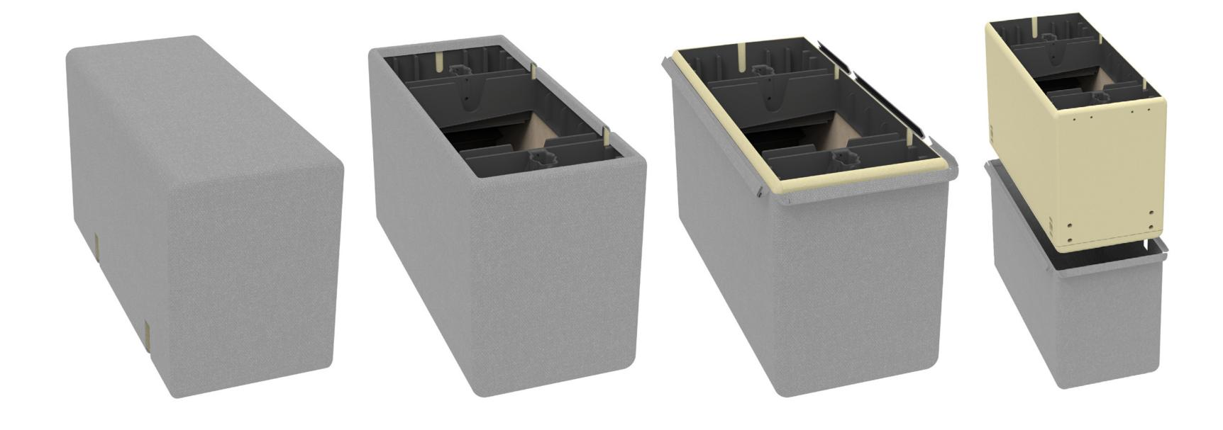
Student life can be hectic, and mess happens! Unlike other seating systems, Exchange's upholstery is not affixed using staples, but with extruded plastic clips sewn directly to the fabric. These clips engage with snap fit details molded directly into the backs, seats and arm rests. If stained or discolored, fabrics can be easily removed and washed, as opposed to discarded.
